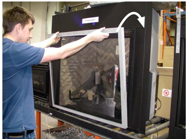
Figure 17d. Pushing screen into place.
