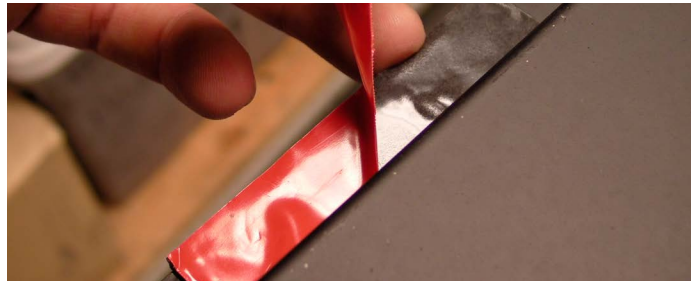
Figure 5.12b Peeling self-adhesive tape
