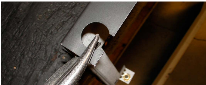
Figure 5.12a Cutting away excess material
