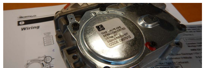
Figure 13.k Conversion label on valve
