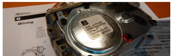
Figure 13.k Conversion label on valve
