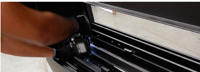
Figure 12.d Removing the Burner screws
