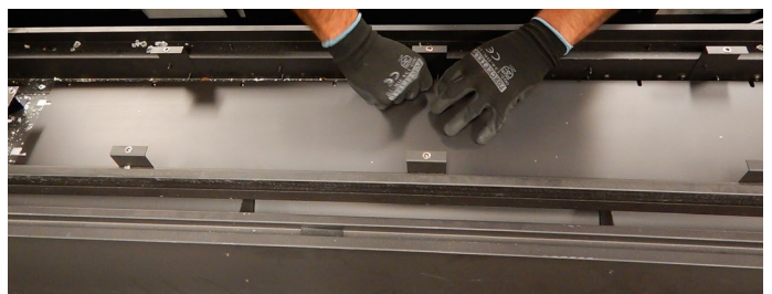
Figure 12.g Removing metal plate
