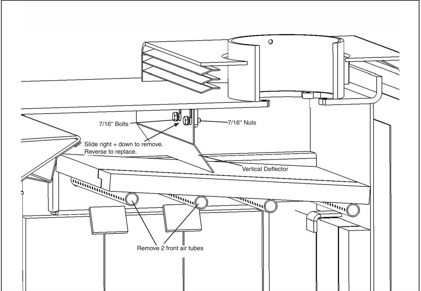
1. Remove 2 front secondary air tubes / vermiculite baffles as per page 21.
