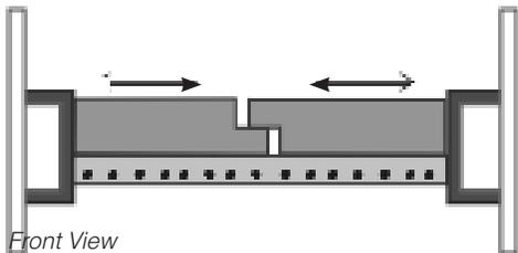
5. Lift the left baffle out from underneath the right baffle - then lift out. Remove the right baffle.
