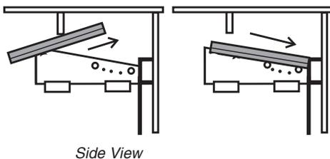
3. Tilt the left baffle up on top of the side channel and it will leave enough room to position the right baffle in the same manner as Step 1) above. Then reposition the left baffle flat on the air tubes.
