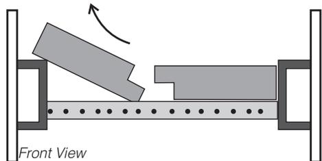
6. Manoeuvre the baffle above the air tube and slide out.
