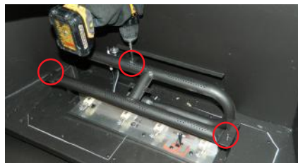
Diagram 2: Slide burner assembly to the right—then remove.
