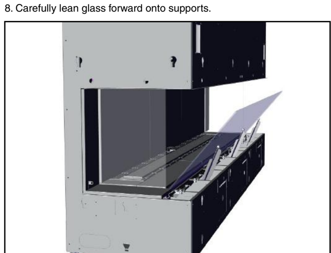
Glass panel--leaning on supports
