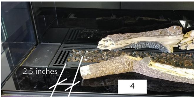
Log 4 to edge of burner
