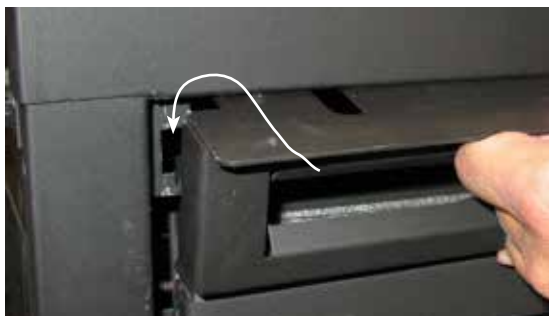
Installation of upper Flush Panel
