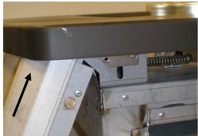
2. Insert Door Face under appliance top and engage lower hooks into slots on face of appliance (See next).
