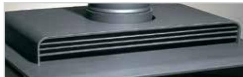
The convector airmate scoops super heated air from the back and top of the stove and directs it to the living area in front. This heat dispersion reduces temperatures behind the unit and allows it to be installed even closer to the wall.
